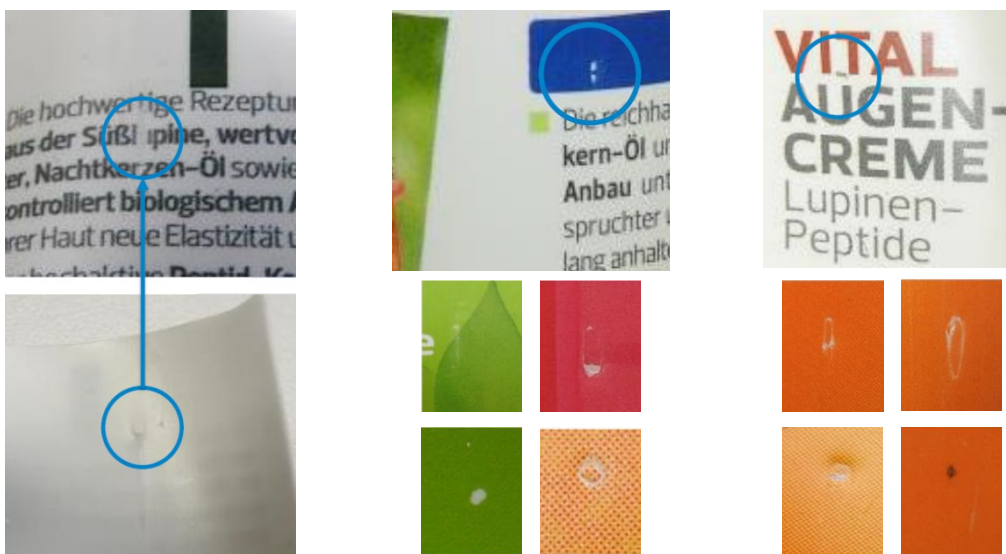
Figure 2: Particles and material inclusions as interfering factors for the decoration on the outside of the tube
